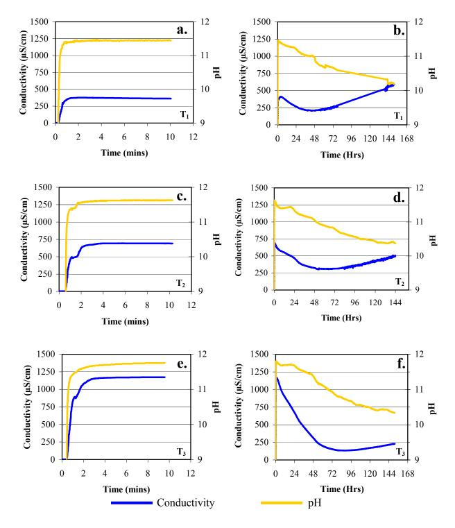
Figure 1a-f: Dissolution plots of 3 calcination grades ( $T_{1-3}$ ) of Enhanced Caustic Magnesia. Plots show conductivity ( $\mu$ S/cm) and pH of a solution containing 10g/L Enhanced Caustic Magnesia. Changes in conductivity reflect the dissolution of the solid Enhanced Caustic Magnesia to form primarily Mg and Ca aqueous species. Rise in pH of the solution is due to the reaction of the Enhanced Caustic Magnesia with water to form Mg(OH)<sub>2</sub> and
