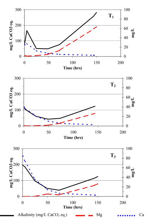
Figure 2: Changes in alkalinity, calcium and magnesium concentrations over time in a solution initially containing 10g/L Enhanced Caustic Magnesia. Experiments with three different calcination grades, low temperature (top), moderate temperature (middle), and high temperature (bottom), indicate that lower calcination temperatures show significantly greater rates of alkalinity release.
