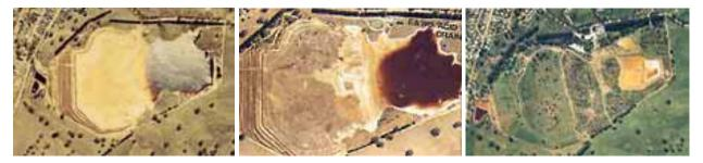
Figure 9. Aerial view of the progressive rehabilitation of the tailings storage facility. Far left: 1973, 12 months after closure of the site. Middle: 1985, remaining acid water on tailings facility after initiation of treatment in 1980. Right: 1997, revegetated surface of the tailings facility.
