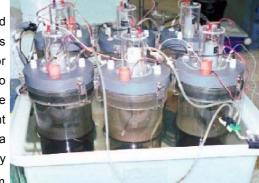
Laboratory testing of nutrient release from sediment cores
